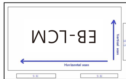
Fig. 2 Reverse scan (Pin24, Reverse = High)
